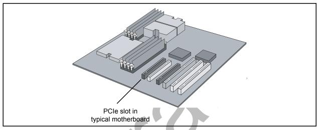
Figure 4-4. PCle Slot in a Typical Motherboard
